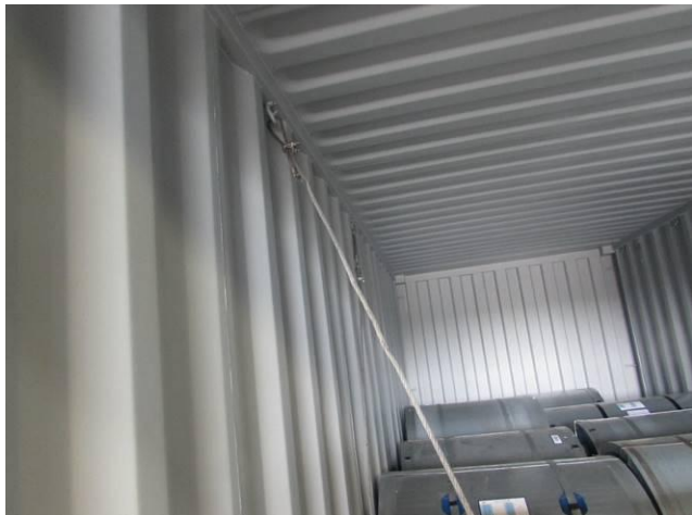
Lashing for front coils.
