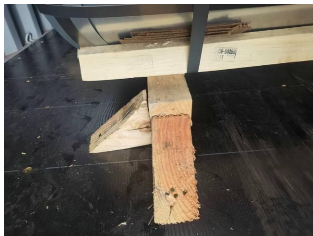
Secured with wire ropes and wedge woods in right side.
