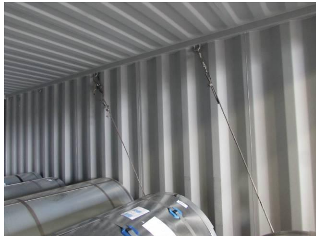
Lashing for front coils.
