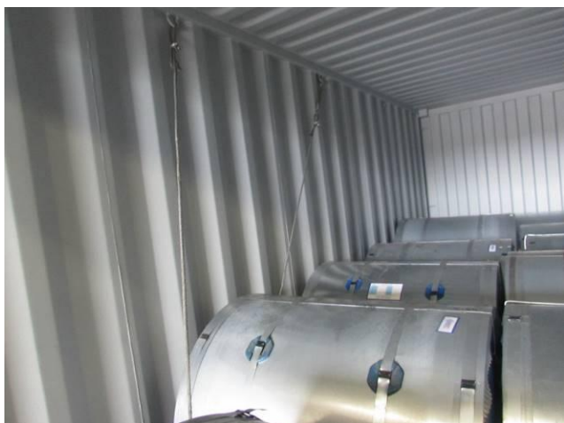
Lashing for front coils.
