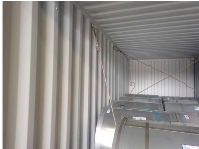
Lashing for front coils.
