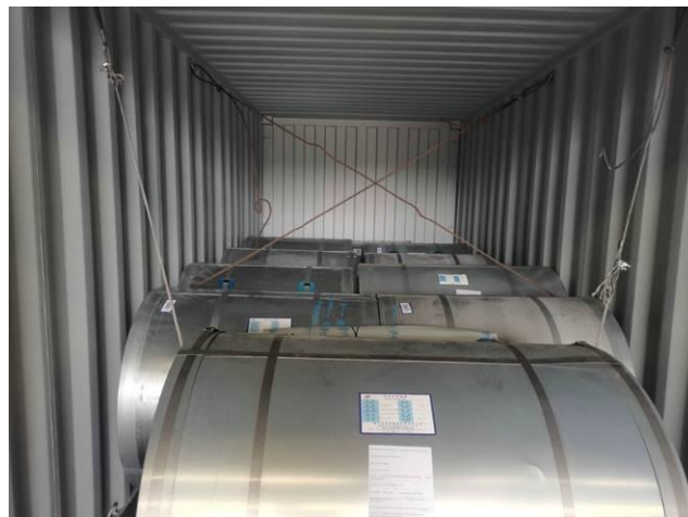
Lashing for front coils.
