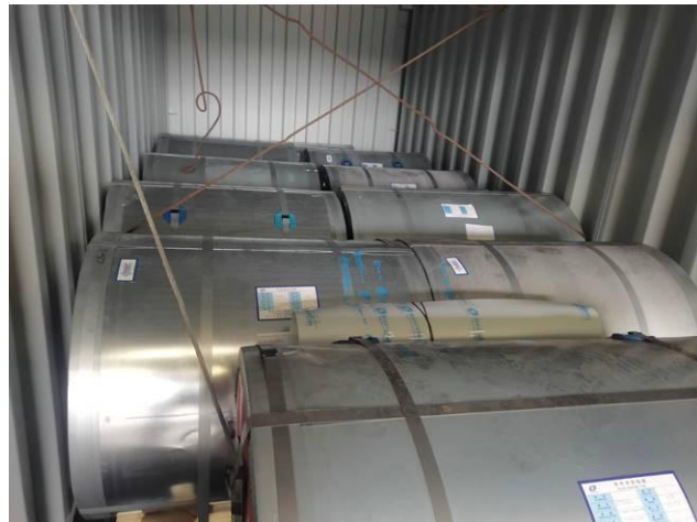
Lashing for front coils.
